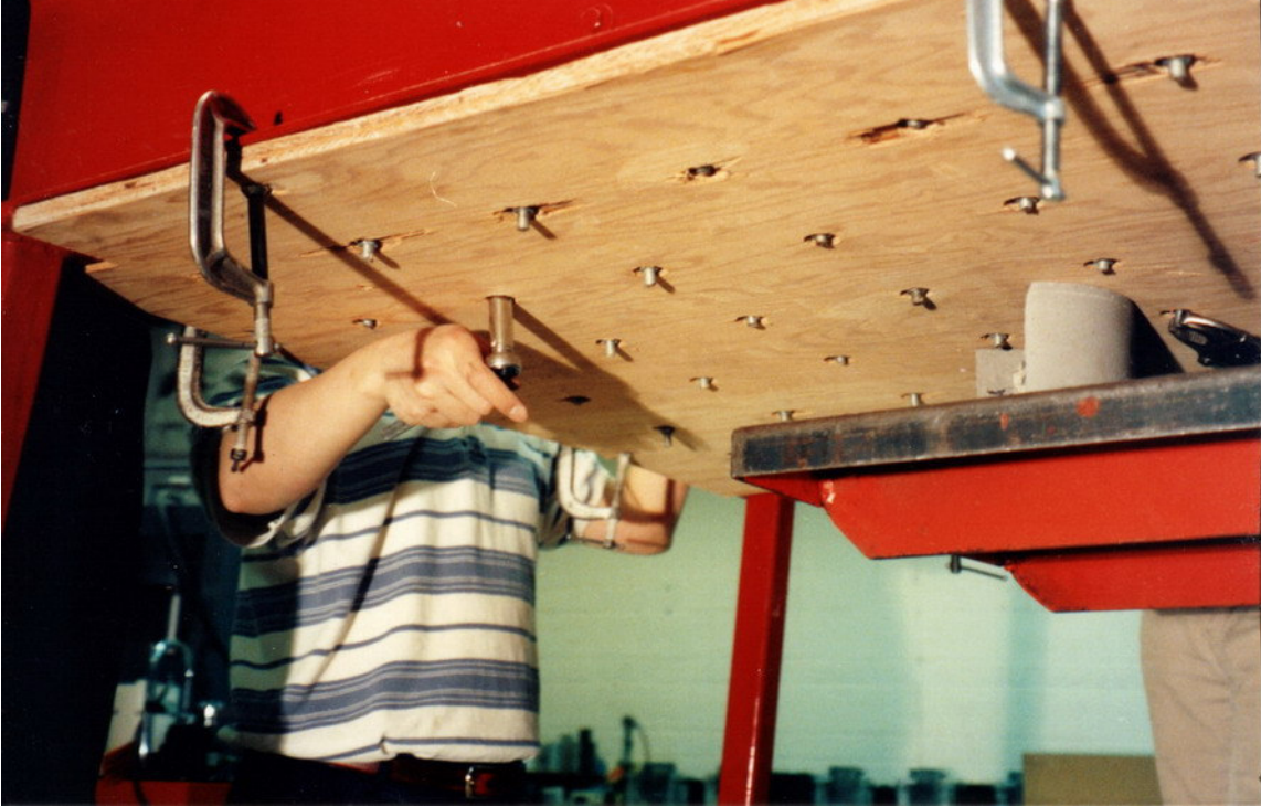
Figure 12: Holding the bottom nut during bolt tightening.
