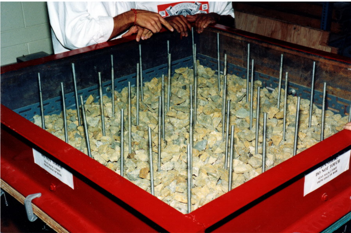
Figure 9: Placing the gravel in the frame.
