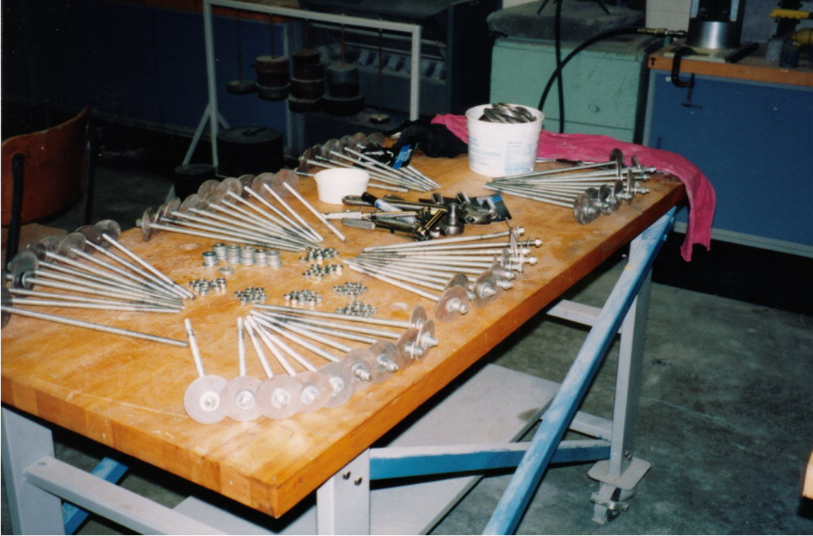
Figure 4: Miniature rockbolts ready for installation.
