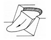
**Failure of Rock Slopes**
